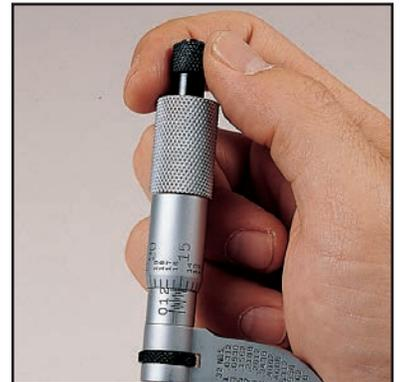
**Ratchet stop/speeder** for consistent measurements and to speed opening or closing of tool.
