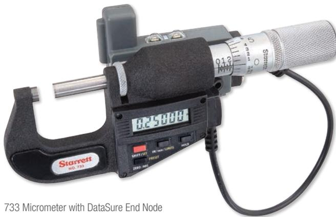
733 Micrometer with DataSure End Node
